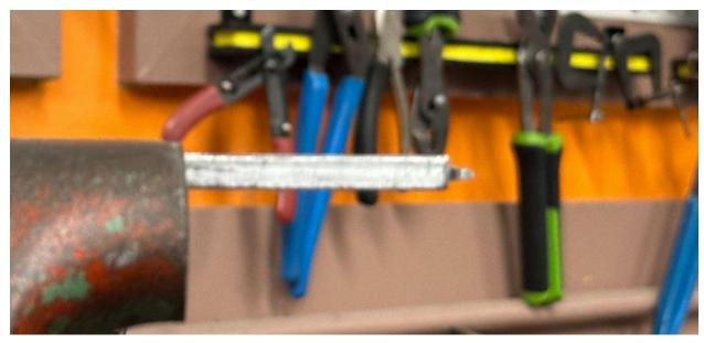
Manual filing for broken edges and refining the flathead rear tip.
