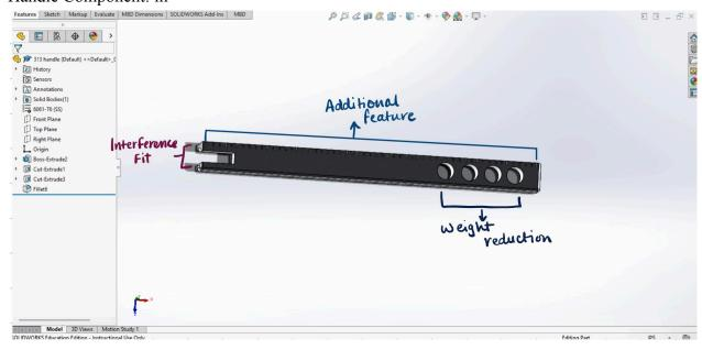
Pictured above is the aluminum handle of this wrench handle design. The three circular cutouts in the handle are designed to reduce the weight without compromising the structural strength of
