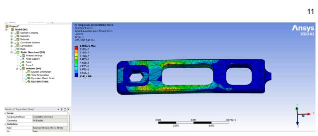
3) 3-point bend test on the handle of 25N: stress, strain, deformation diagrams
